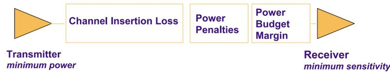
$$\text{Link Power Budget} = \text{Min transmit power} - \text{Min receiver sensitivity}$$
