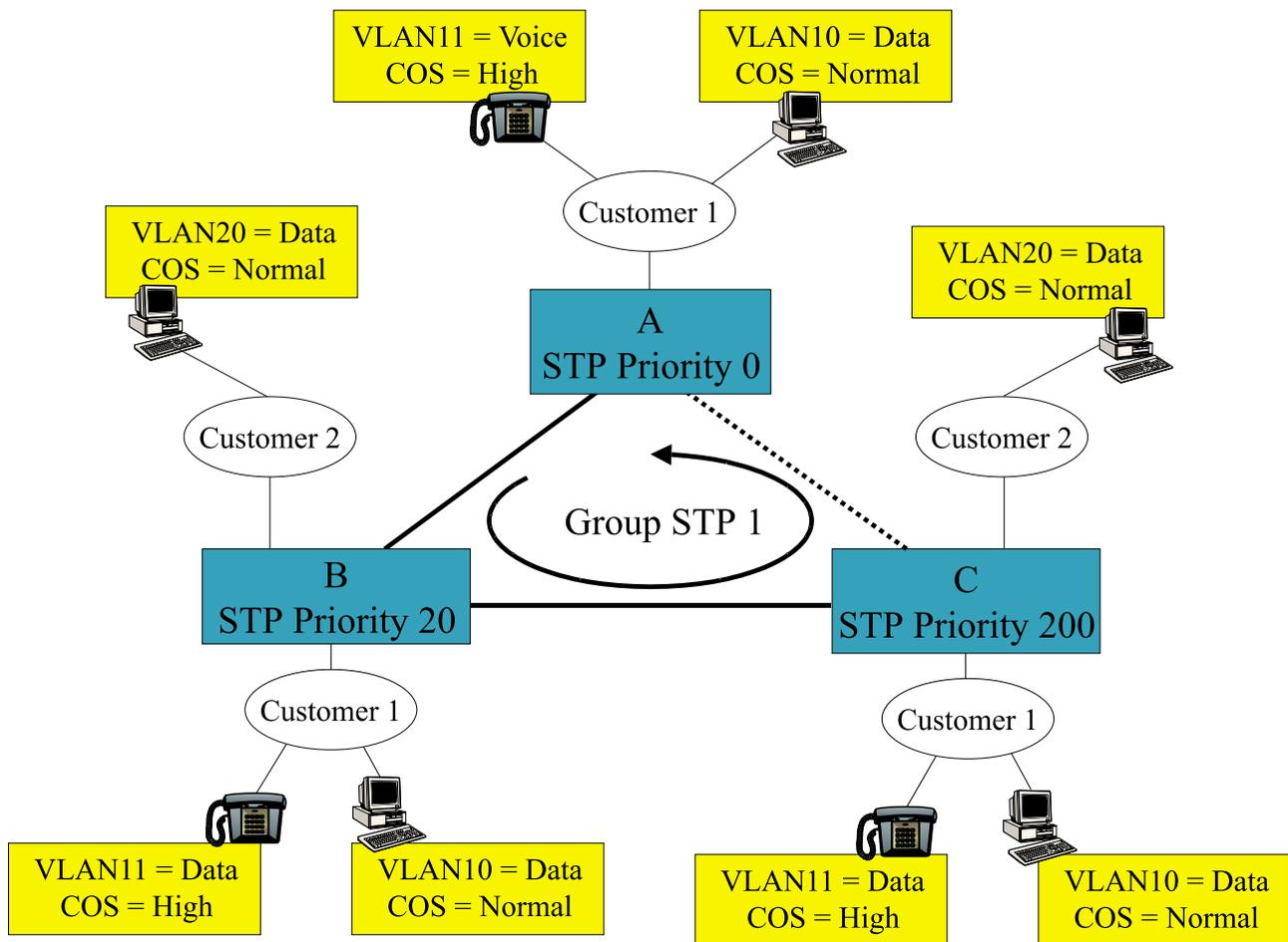
Figure – 9: Delivering Service Differentiation Within Ethernet..
