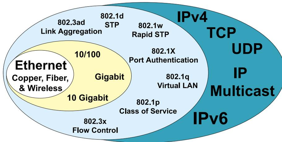
Figure - 1: Various Standards that Work with Ethernet.
